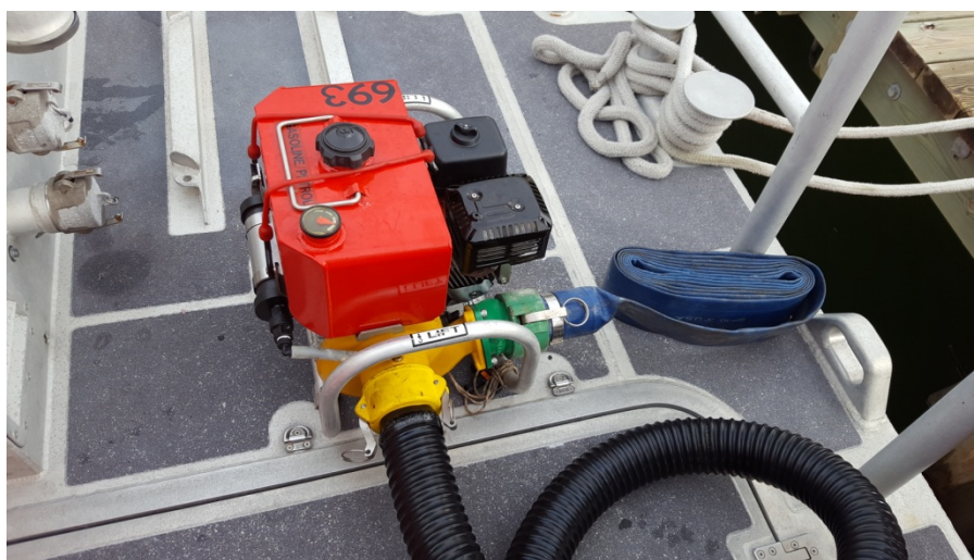
Figure 5-6 Drop Pump Readied for Dewatering Action
