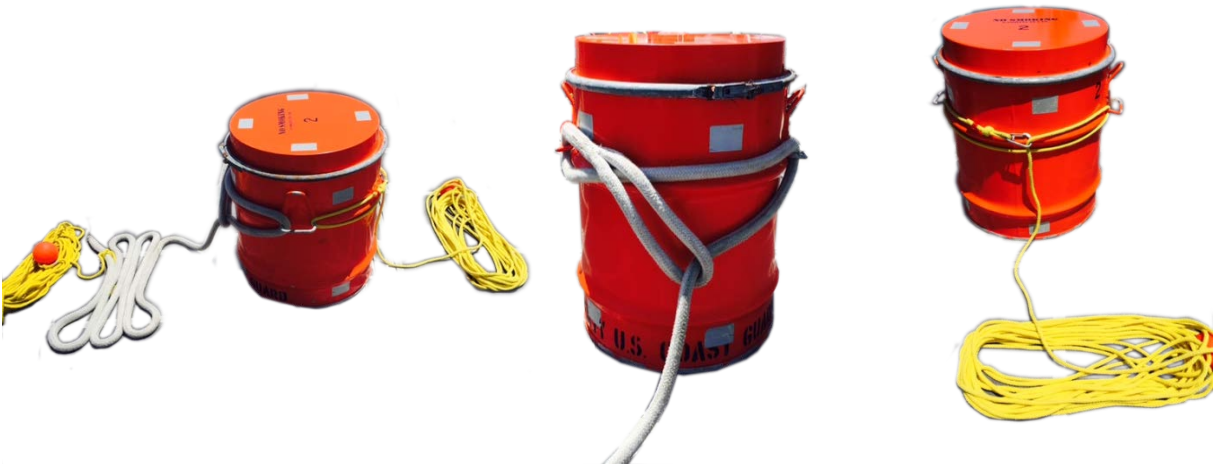
Figure 5-7 Securing Lines to Drop Pump Container
