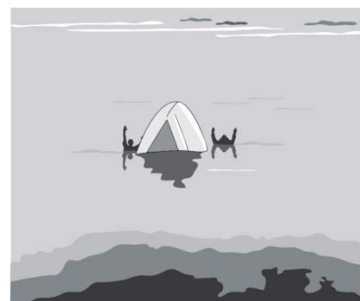
Figure 2-4 Black Hot Thermal Display
