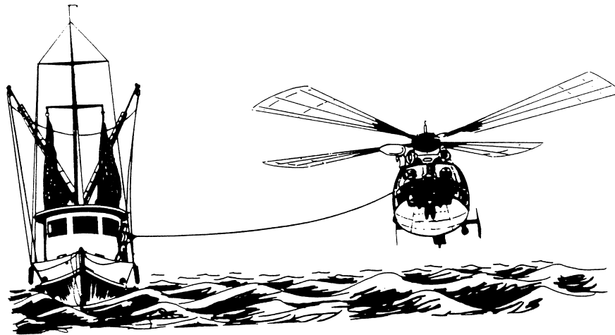
Figure 6-13 Indirect Delivery of Pump
