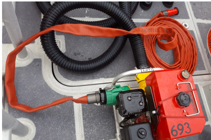
Figure 5-19 CG-P6 Pump With Fire Fighting Hose and Nozzle Attachments
