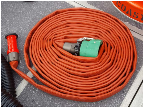
Figure 5-15 Fire Fighting Hose
