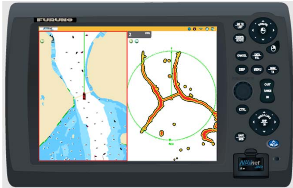
Figure 3-17 Multi-Function Display / Electronic Chart Plotter (Example)
