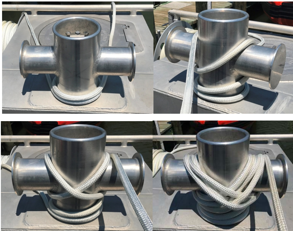
Figure 2-35 Securing a Line to a Single Bitt
