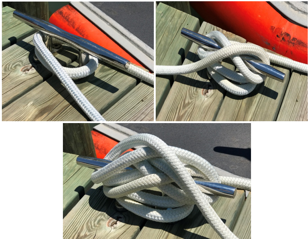
Figure 2-36 Securing a Line to a Cleat
