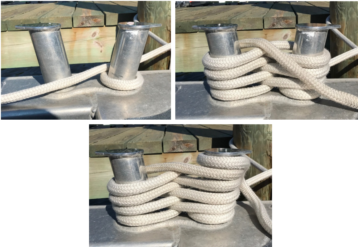
Figure 2-34 Securing a Line to Paired Bitt
